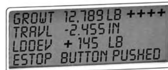
OPERATE Mode E-STOP Button Pushed
