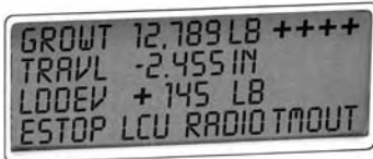
OPERATE Mode showing E-STOP for Radio Timeout
